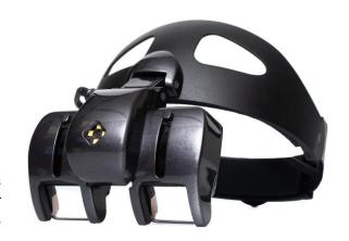
micro-displays and beam splitter plates. As two displays are available, one for each eye, a three-dimensional content can be visualized by utilizing the stereoscopic effect in the natural field of view of the user.
